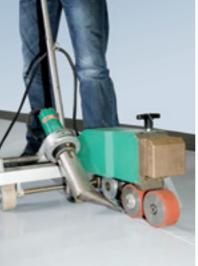
Fig. 5: welding with the hot air welding machine
